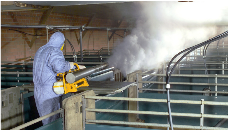
Use of the portable thermal fogger pulsFOG K-22/O
